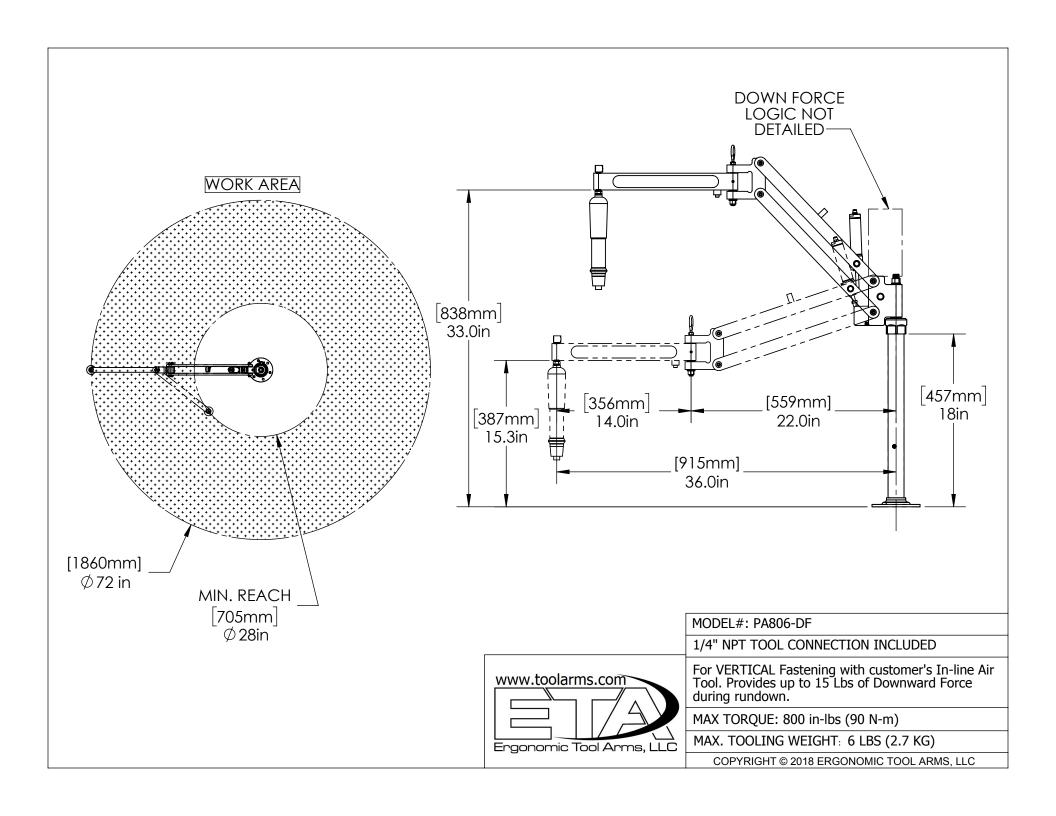
For operations that require the assembly personnel to provide downward thrust to successfully drive screws, the ETA arms with DOWN FORCE ASSIST (DF Models) can transform the production process. Sometimes it can be very fatiguing to drive self-threading fasteners, self-drilling screws or fasteners with lock-patches or nylon inserts because it requires so much downward force to keep the driver bit engaged in the head of the screw.
