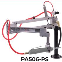
Standard-duty arm for Inline or Pistol Air Tools fastening Horizontally. Included PS holder keeps tool horizontal while spinning for axial alignment with horizontal fasteners. Maximum torque is 275 in-lbs (31 Nm) on this model with a maximum tool weight of 4.8 lbs (2.16 Kg). 5/16" ID tool supply hose included. See our website for similar arms with other capacities using the PS and PT holders.
