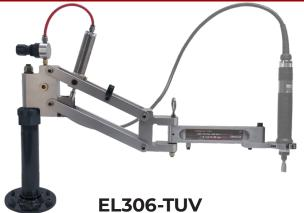
Standard-duty arm with a compact design for shorter reach than 506 arms. Ideal for assembly of smaller parts and tighter work areas. This model includes the thinner TUV holder for Inline Electric Tools 1-1/8" (28.6mm) to 2.0" (50.8mm) in diameter fastening Vertically up to 550 in-lbs (62 Nm) with a maximum of 5 lbs (2.25 Kg) of tool weight. See our website for similar arms with higher capacities.
